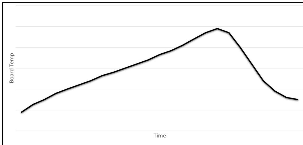
**Figure 3: Example of a Ramp to Soak to Peak Profile (RSP)**
