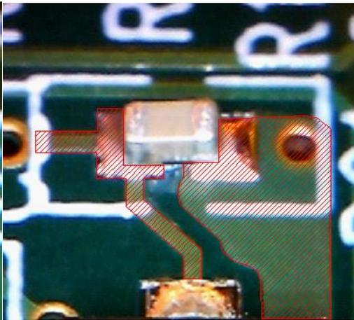
The test vehicle is a multilayer PCB with Electroless Nickel Immersion Gold (ENIG) surface finish. This assembly was chosen for the test because of tombstoning and open defects, resulting in an unacceptable Defects per Million Opportunities (DPMO) on 0402 components.
